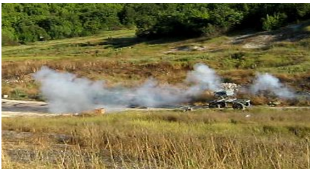
Pict. 5. Pulse pulverization of 2,5 kg bio-sorbet out of single barrel to range 15 m, wide uniform cover 1–3,5m 2 along trajectory of pulverization and area of uniform cover is 35–45m 2
