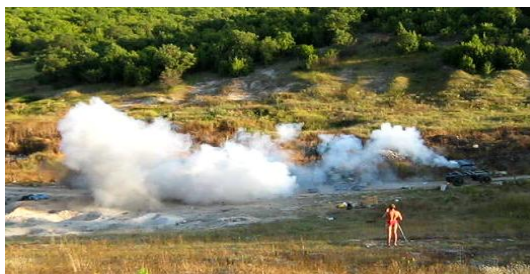
Pic. 4. Volley with 5 barrels, pulverized 12,5 kg biosorbents to range up 55 m, wide of uniform cover 2–10 m along the trajectory and area of uniform cover to 450 m 2
